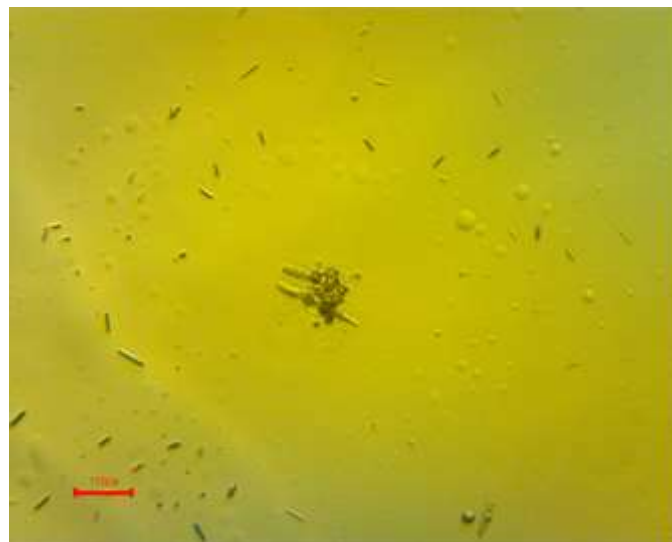
Figure 3.24. Graphene scrolls or spicules dumped at the bottom of the slide.
