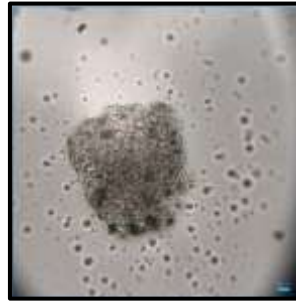
Figure 3.4. Microcrystalline Calcite with graphene inclusions.
